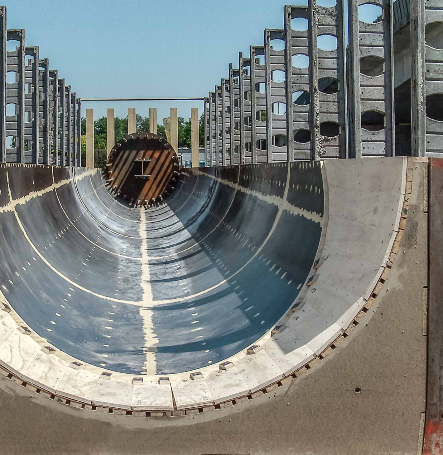
Special formwork made of wood for the production of prefabricated components.
