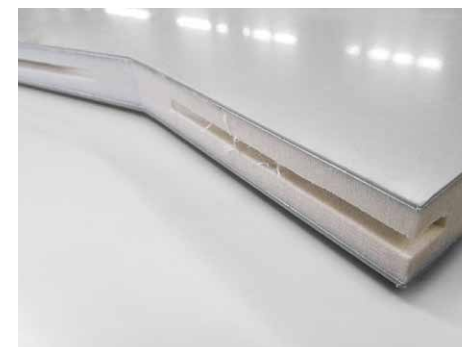
Milled, butt jointed and then connected with Lamello connectors without welds.
