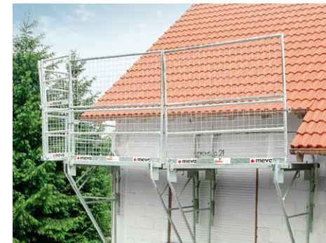
Vertical extension of the guard railing also allows the LAB 130 working platform to serve as a fall-arrest scaffold below the roof.
