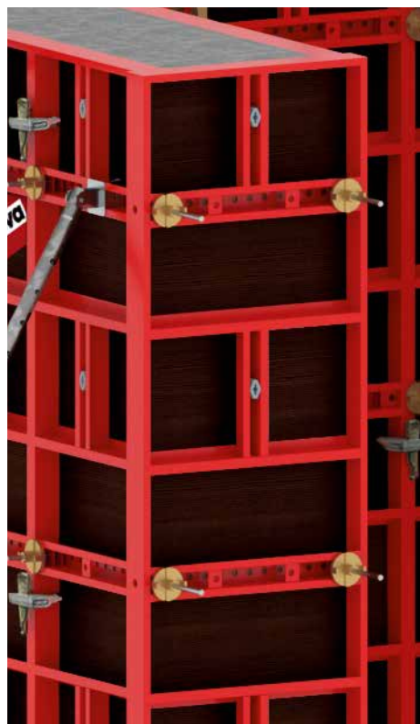
55 cm width standard EF panel for up to 25 cm width walls. 75 cm width standard EF panel for up to 45 cm width walls.
