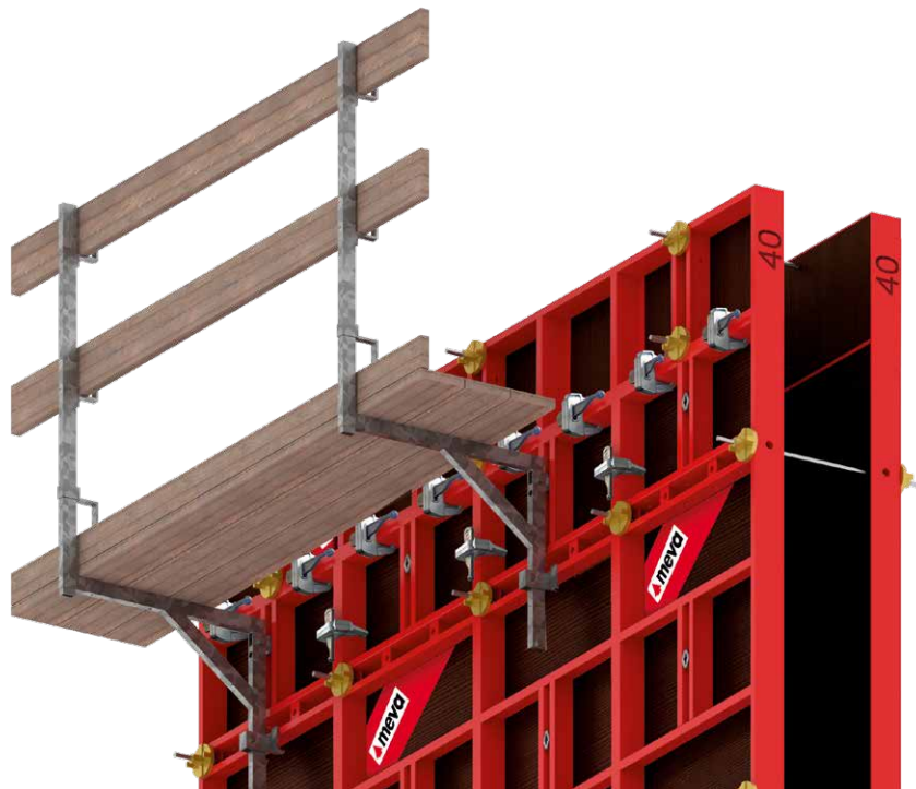
When a EF panel of less than 55 cm in width is horizontally stacked on a vertical EF panel, the Walkway Bracket is fixed onto the vertical panel.
