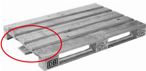
A block is missing or split in such a way that more than one nail shank is visible.
